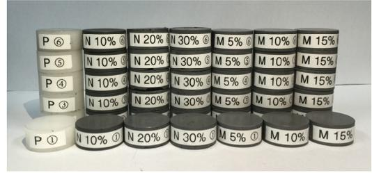
Fig. 2 Specimens for compressive strength test.
