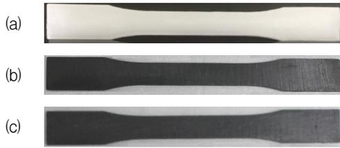
Fig. 1 Specimens for tensile test: (a) pure paraffin wax, (b) w/ nano size aluminum (c) w/ micro size aluminum.
