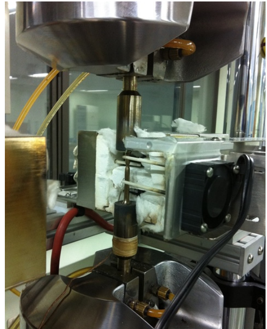
Fig. 2 High temperature chamber and extensometer of tensile test system.
