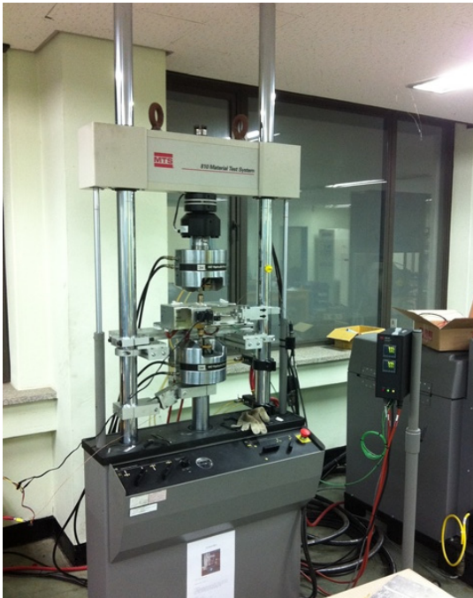
Fig. 1 Hydraulic high temperature tensile test system (MTS).
