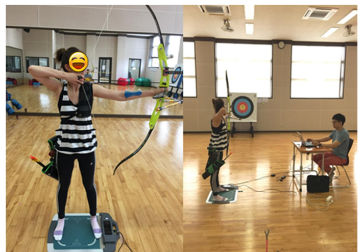
Figure 3. Analysis of foot plantar pressure in dynamic balance during shooting.
