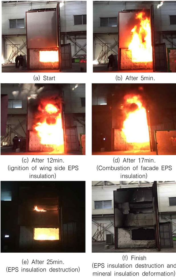
Figure 7. Fire test result as elapsed time
