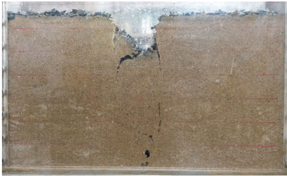
Fig. 5 Typical Cavity Expansion in Unsaturated Sand
