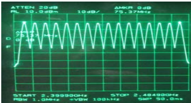
Figure 11: RF Channel and the Power Level Measurement
