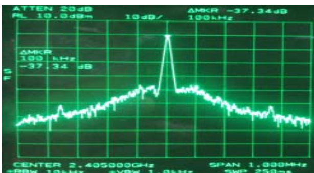
Figure 13: The P/N Characteristic in 100 kHz Offset
