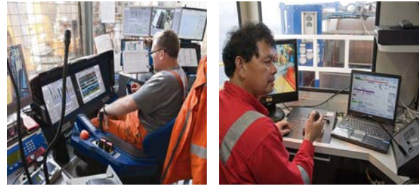
Figure 6: Cyber base(Driller cabin)
