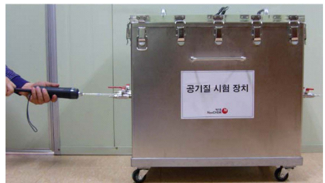
Figure 2. Illustration for gas removal test with dark chamber.
