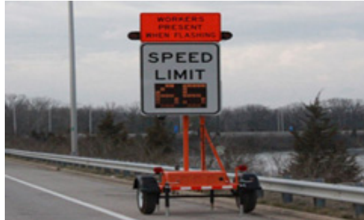
Figure 7. Example of PVMS+VSL in work zone
