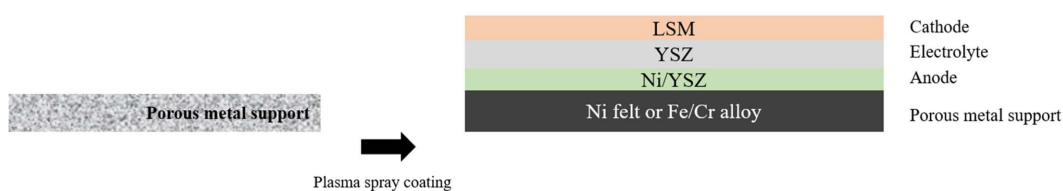
Fig. 4. DLR fabrication process for metal supported cell.
