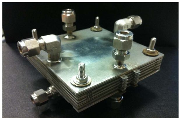
Fig. 13. A 50 \text{ mm} \times 50 \text{ mm} metal-supported five-layer stack.
