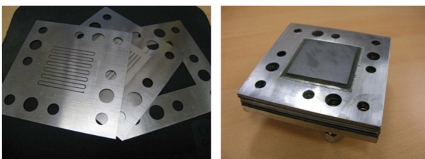
Fig. 9. Metal-supported SOFC bipolar plate (left) and a 5 \times 5 \text{ cm}^2 stack (right).
