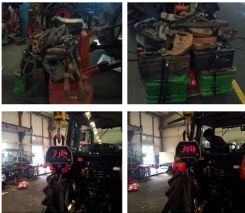
Fig. 5. Photo of the hydraulic capacity test.
