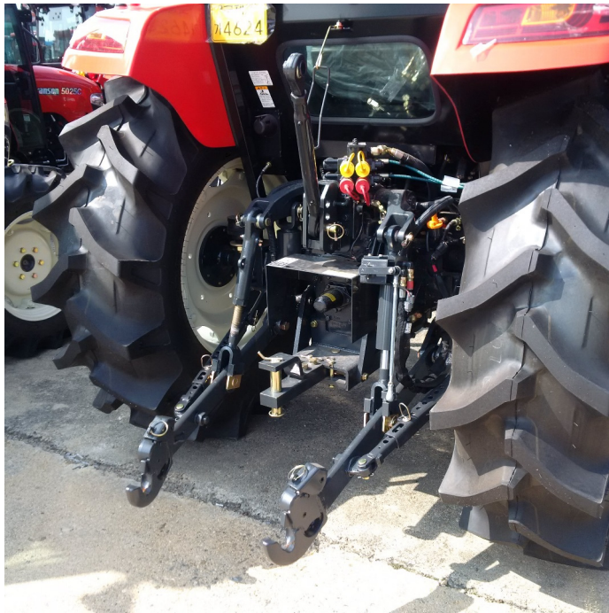
Fig. 7. Photo of the 3-point hitch developed in the study.
