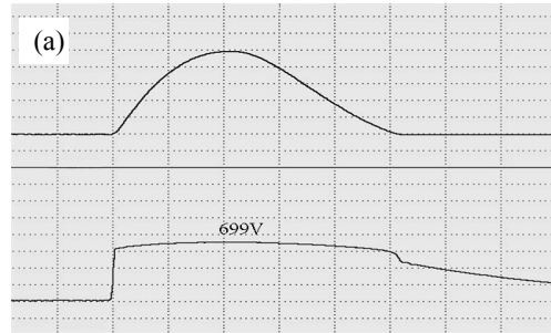
Upper : impulse current [100 V/div, 5 μs/div] Lower : clamping voltage [100 A/div, 5 μs/div]
