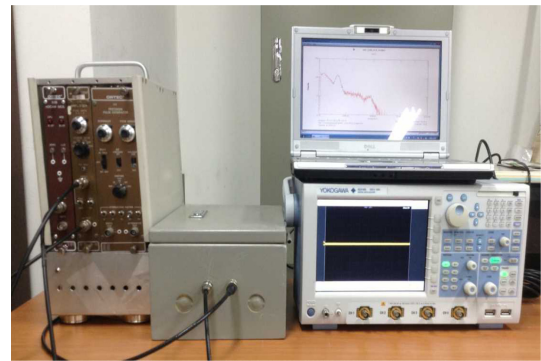
Fig. 2. Experimental setup for measuring beta-ray detection efficiency.
