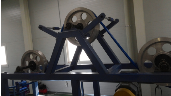
Fig. 11. Fatigue test equipment for bending and tension
