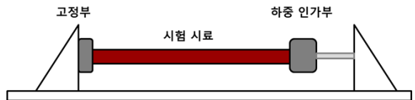
Fig. 10. Test setup of cable break load
