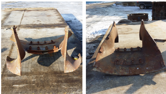
Fig. 4. Damaged blast door after testing
