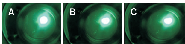
Fig. 4. FEM image structure for emitter 1, at emission current 1.5 μA, and applied voltages: (A) 2,400 V, (B) 2,300 V, (C) 2,200 V. Time separation between consecutive images is 15 minutes.
