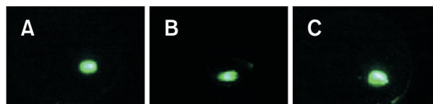
Fig. 8. FEM image structure for emitter 3, at emission current 1.4 μA, and applied voltages: (A) 1,500 V, (B) 1,400 V, (C) 1,300 V. Time separation between consecutive images is 15 minutes.
