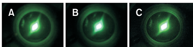
Fig. 6. FEM image structure for emitter 2, at emission current 1.5 μA, and applied voltages: (A) 1,500 V, (B) 1,400 V, (C) 1,300 V. Time separation between consecutive images is 15 minutes.
