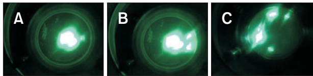
Fig. 12. FEM image structure for emitter 5: (A) 1.5 \mu\text{A} at 9,700 \text{ V} ; (B) 6.8 \mu\text{A} at 9,600 \text{ V} ; (C) 6.8 \mu\text{A} at 9,300 \text{ V} . Time separation between consecutive images is 15 minutes.
