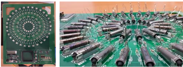
Fig. 7. Experimental Device for 48 Channel GM Tube Sensor Test.
