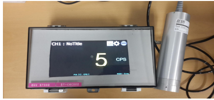
Fig. 4. Operational screen shot of the Stack Monitoring System
