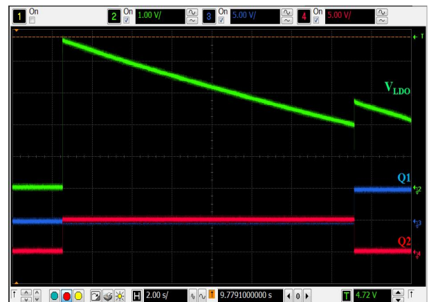
Fig. 10. LDO input voltage of a conventional SCALDO regulator (5V to 2V, I_{out}=300mA )
