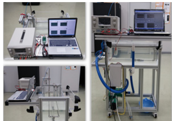
Fig. 4 Experimental apparatus of velocity sensor evaluation under electrolyte flow in electroplating bath
