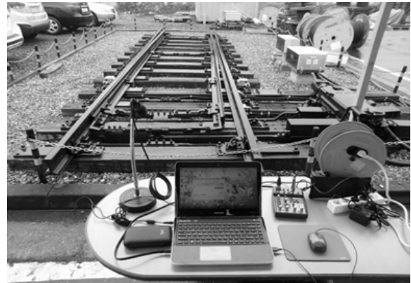
Fig. 5. Data collection from railway point machine
