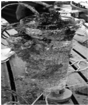
Fig. 2. Damaged Underwater Sensor by fouling[11]
