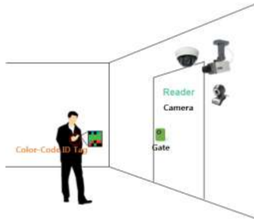
Figure 2. Color Code based Gate Access Control System
