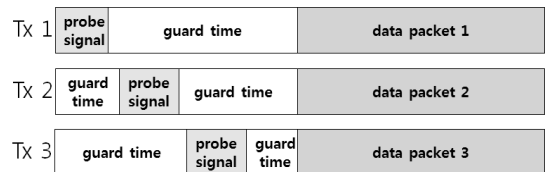
Fig. 4. The transmitted signal packet structure.
