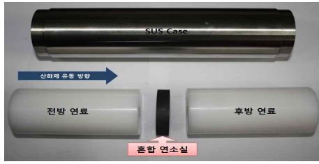
Fig. 2 Configuration of Fuel Grain
