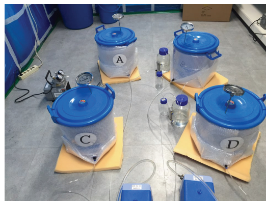
Swine manure composting reactor
