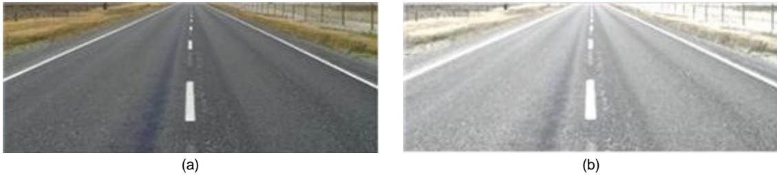
Fig. 3 Gaussian filter image (a) Original image (b) Image applied Gaussian filter
