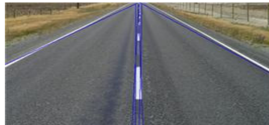
Fig. 7 Lane detection result with Hough transform
