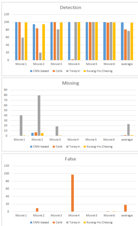
Fig. 11 Comparison of CNN-based fire detection with previous studies
