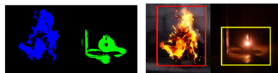
Fig. 10 ROI extraction using labeled masks
