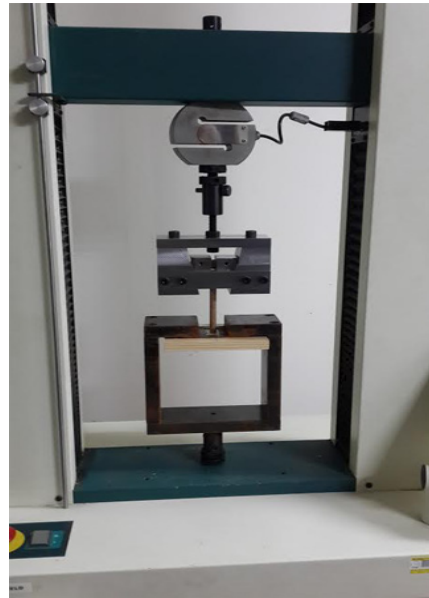
Fig. 1. Test setup for dowel withdrawal load.
