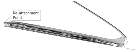
(a) Streamlines in neutral posture at v = 30 m/s
