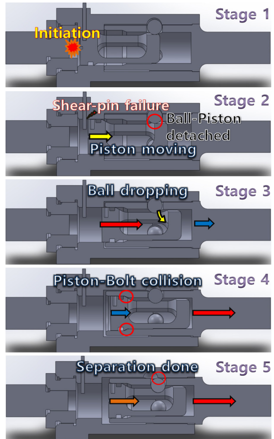
Fig. 5 Stage modeling of separation behavior based on AUTODYN analysis results.
