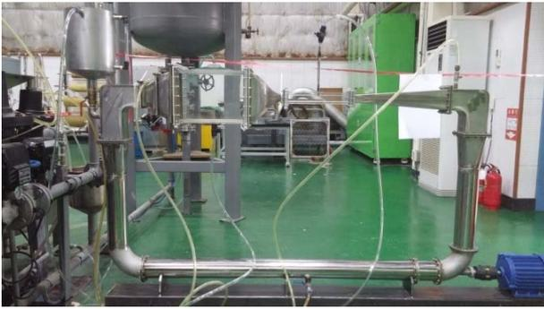
Fig. 8 A tenth miniature model of the medium-sized high speed tunnel
