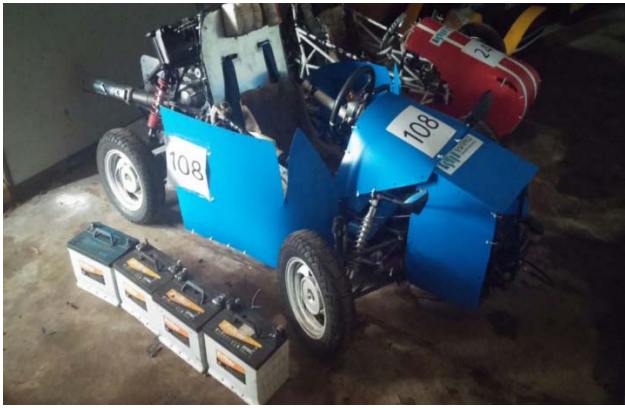
Fig. 7. Four valve-regulated lead–acid batteries used for SOH investigation.
