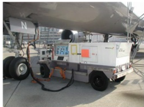
Fig. 10. GPU for electrical power [11]
