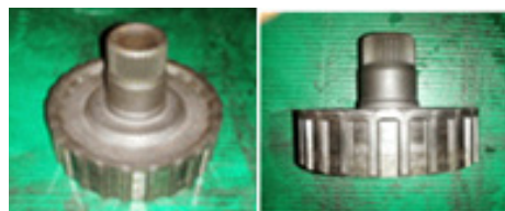
Fig. 3. Reaction hub of automatic transmission
