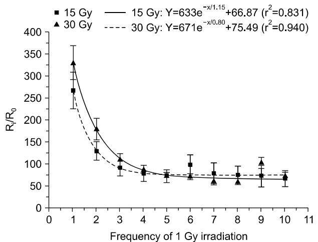
Fig. 5. The change of residual count of high dose irradiated OSLDs by repeated irradiation with 1 Gy. Each data point is the average response of three individual dosimeters.
