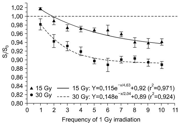
Fig. 4. The change of relative radiation sensitivity of high dose irradiated OSLDs by repeated irradiation with 1 Gy. Each data point is the average response of three individual dosimeters.
