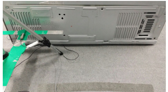
Fig. 7 Location of the microphone for the error sensor
