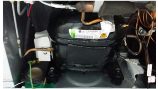
Fig. 2 Reference sensor on the shell of the compressor and the control speaker next to it
