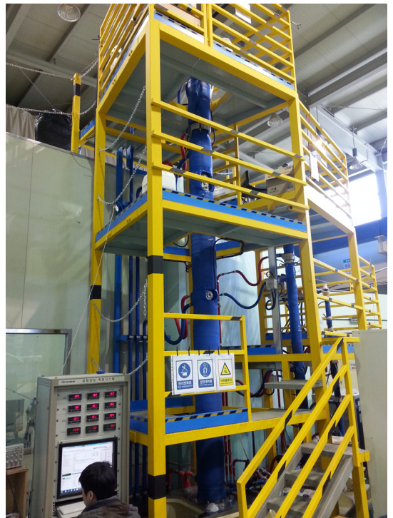
Fig. 4 Underwater acoustic performance measurement system(pulse tube)
