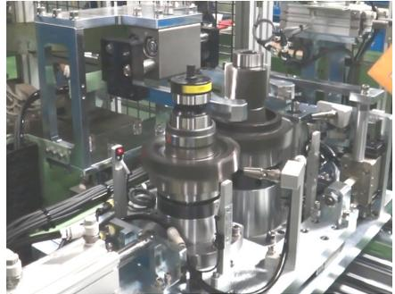
Fig. 6 Transmission error measurement system
