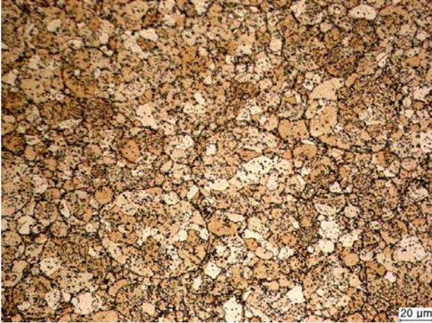
Fig. 1 Microstructure of hot isostatically pressed nickel superalloy using optical microscopy
