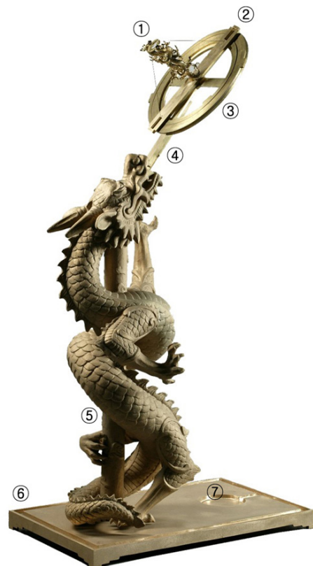
Fig. 1. Sun-and-Stars Time-Determining Instrument reconstruction model (National Folk Museum of Korea) designed by Needham et al. (1986). ① pole-fixing ring, ② an alidade, ③ three rings, ④ a wheel and handle, ⑤ a dragon column, ⑥ a stand, and ⑦ a pool.
