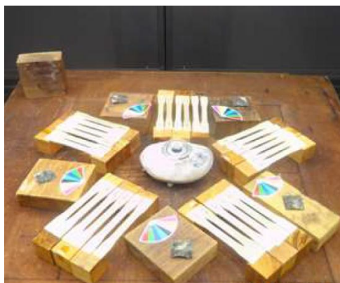
Fig. 4. Specimen arrangement for solar radiation test
