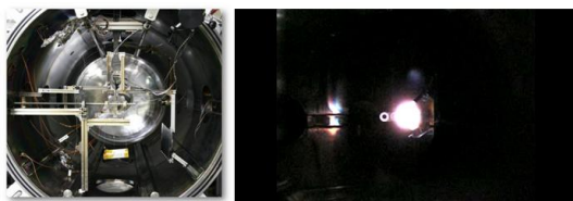
Fig. 7. Ion Thruster Discharge Test
