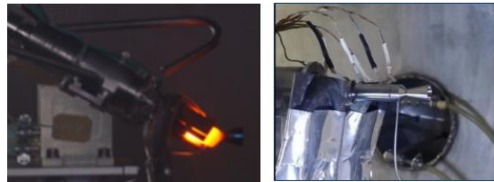
Fig. 2. 5 N / 1 N Class Hydrazine Thruster
