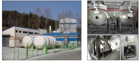
Fig. 1. Long Life Firing Test Facility for Hydrazine Thruster
