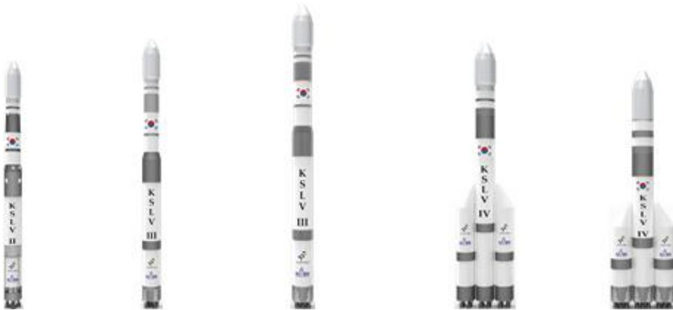
Fig. 1. Concepts of launch vehicles using multi-engine clustering and common booster core
