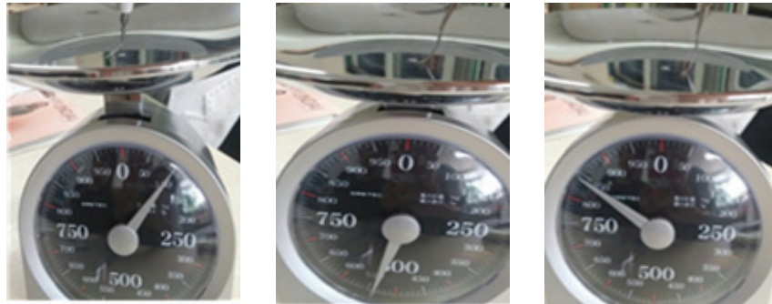
Fig. 3. Lateral pressure measurement using the weighing scales
