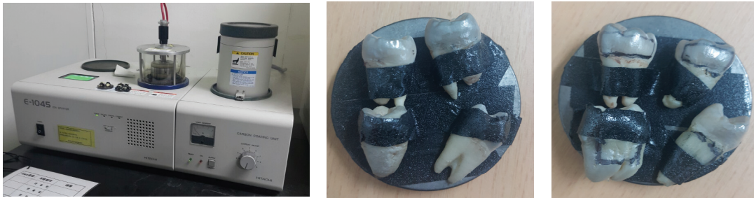
Fig. 2. Test specimen coated with equipment(Hitachi E-1045)
