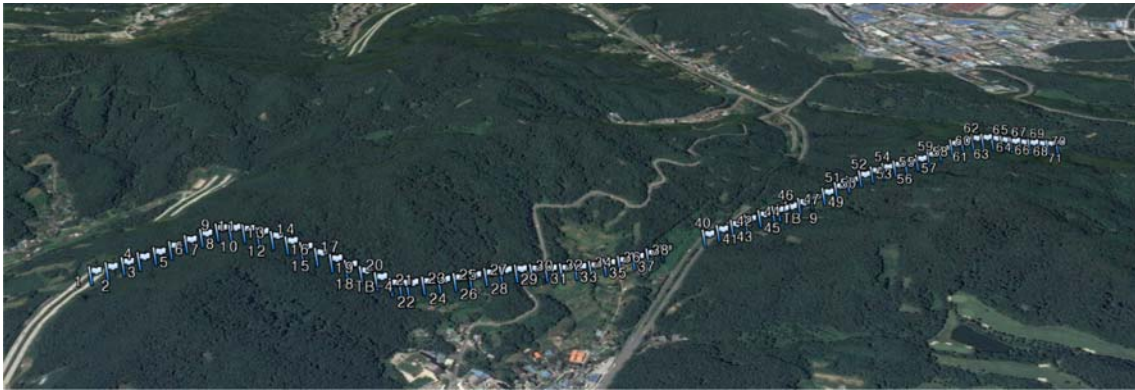
Fig. 6. Overview of survey line and marked station numbers for seismic tomography. The line crosses 2 roads and the elevation range is 141 m to 304 m (Google Earth).
