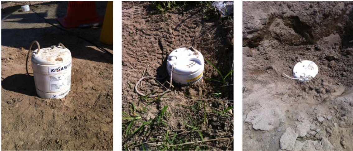
Fig. 3. 3 types of node deployment. The node depends on the condition of the surface and needs tight coupling for reducing noise.
