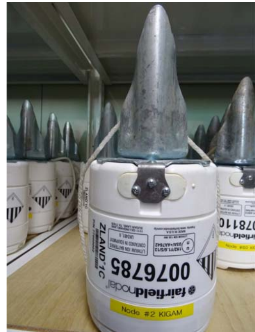
Fig. 2. A cable-free receiver which has 10 Hz natural frequency geophone with sensitivity of 80 V/m/s, GPS unit with 2.5 m accuracy and timing accuracy 99% less than 60 ns, 8 GB memory, and Li-Ion battery.
