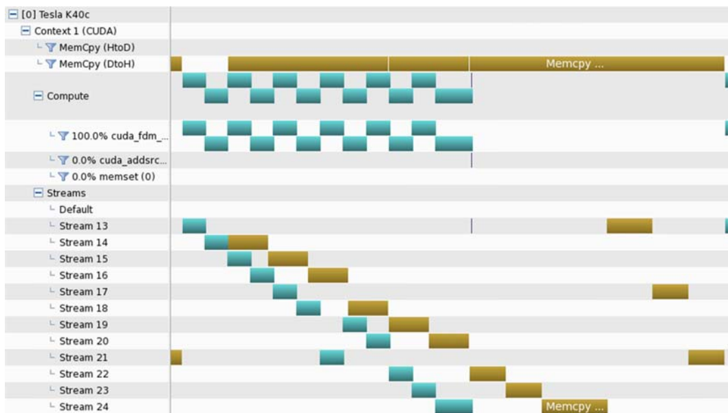
Fig. 4. A screenshot of a GPU profiling tool showing one time iteration. Green boxes show the finite difference calculation processes and yellow boxes show the memory copy processes. The width of a box shows duration of that process. There are 12 streams and a calculation process in one stream can be overlapped with a memory copy process of another stream. Note that the time of the memory copy process takes most of the execution time.
