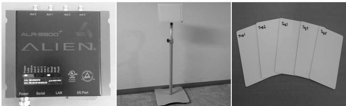
Fig. 1. Views of the ALR-9900 + RFID reader, MT-92 antenna and ALN-9629 passive tags used in this study
