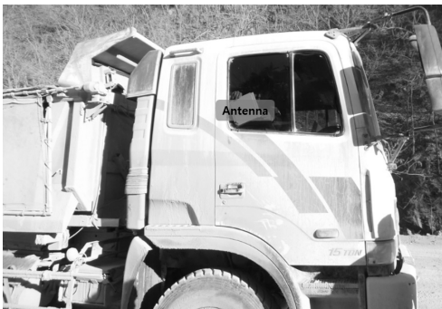
Fig. 6. Reverse RFID system mounted on dump trucks in the study area
