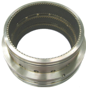
Fig. 5 Assembly of the honeycomb seal
