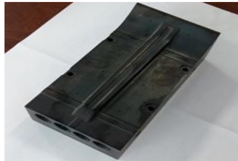
Fig. 6 MBR upper mold after heat treatment
